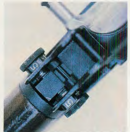
ABOVE: Rear sight assembly on Type 81 rifle provides a realistic maximum elevation of 500 meters. Note retracting handle, which resembles that of the SKS.
